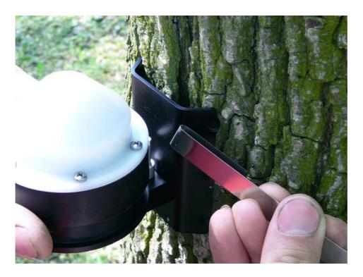
3/ Wrap the tape around the stem and than wrap it around the coil
