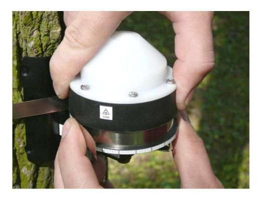
7/ The tape has to remain under tension – check the scale position (> 0).
