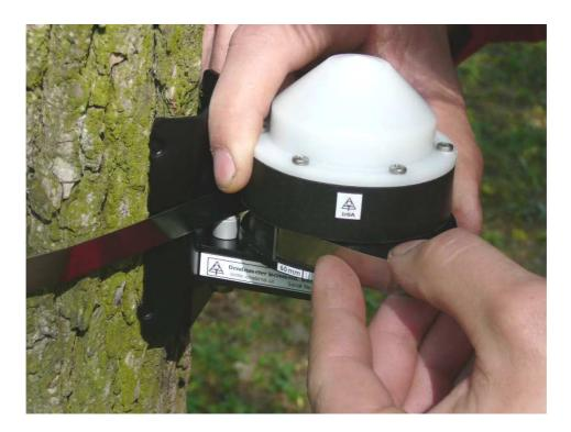
5/ Turn the head counterclockwise in order to get at least 5 mm on the scale
